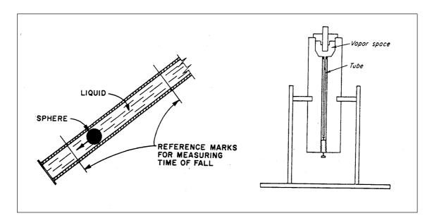
Fig. 4.4: Schematic diagram of the falling ball viscometer.
