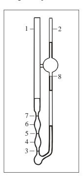
Fig. 4.6: Viscometer apparatus.
