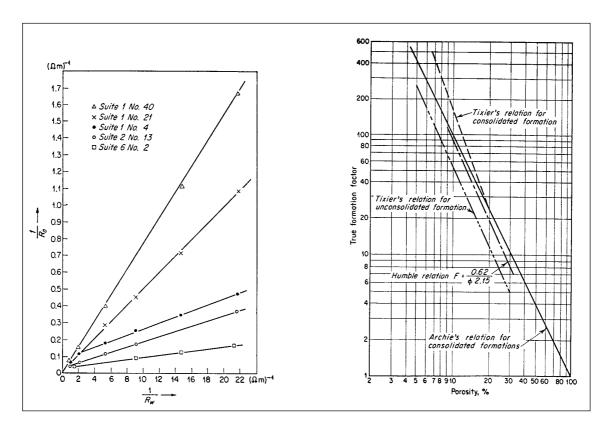
**Fig. 6.2:** Water-saturated rock conductivity as a function of water conductivity.
