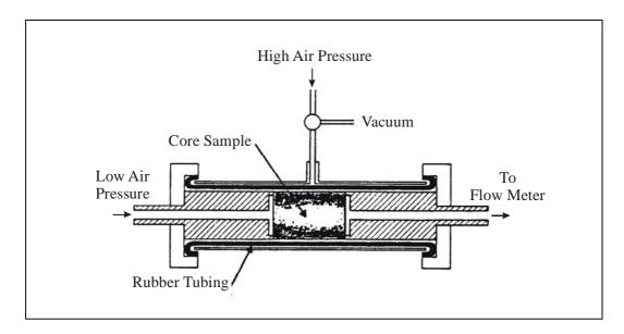
**Fig.10.4:** Hassler type core holder.
