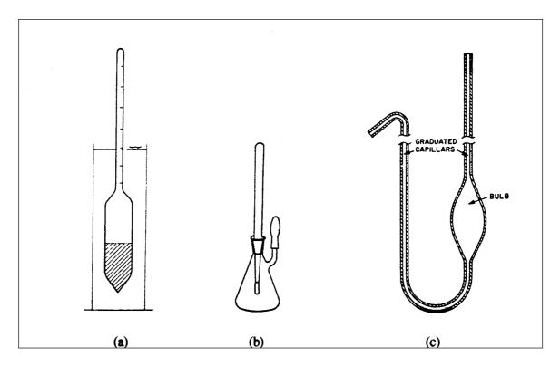
**Fig. 3.1:** Schematic diagram of hydrometer (a), pycnometer (b), and bicapillary pycnometer (c)
