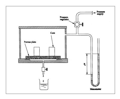
**Fig.9.7:** The capillary pressure apparatus.
