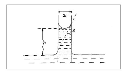
Fig. 7.2: Capillary-rise method.
