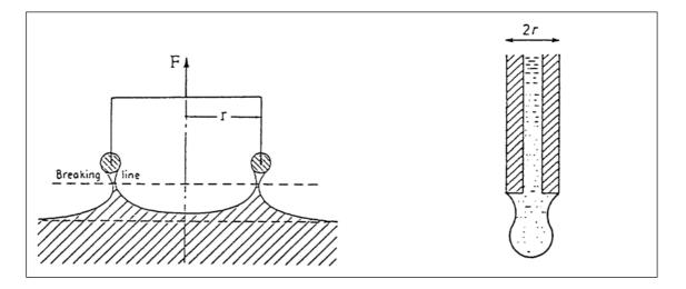
**Fig. 7.4:** Ring method. **Fig. 7.5:** Hanging drop from a capillary tube.
