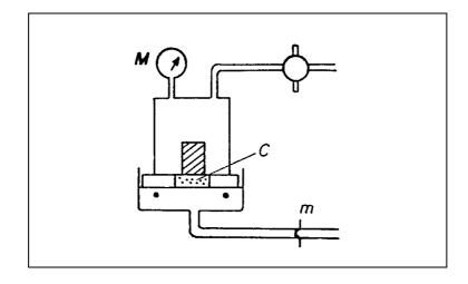
**Fig. 9.2:** The porous plate method assembly.
