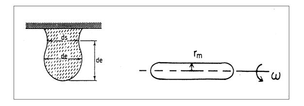
**Fig. 7.6:** Relationship between dimensions of a pendant drop.
