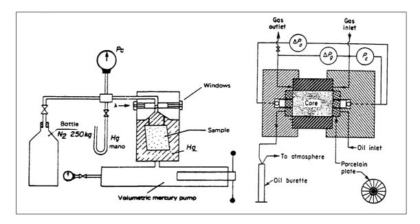
**Fig. 9.5:** Apparatus for mercury injection method.
