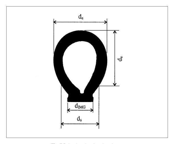
Fig. 7.8: Pendant drop imaging picture.
