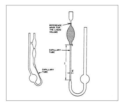
Fig. 4.3: Two types of Ostwald viscometers.
