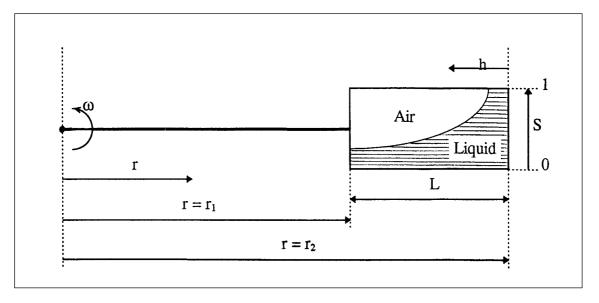
Fig. 9.3: Schematic diagram of a core in a centrifuge and its boundary conditions.
