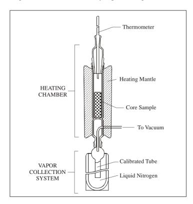
Fig. 2.2: Vacuum distillation Apparatus.
