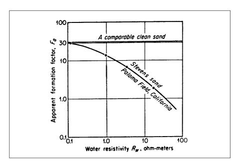
**Fig. 6.1:** Apparent formation factor versus water resistivity for clayey and clean sands.
