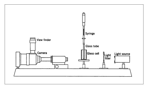
**Fig. 8.4:** The image system set-up.
