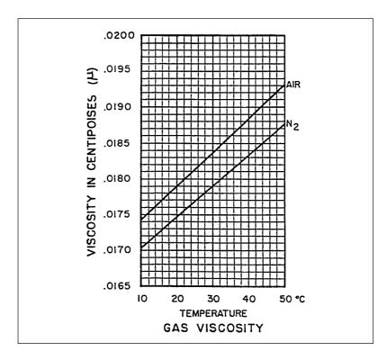
Fig. 10.5: Gas viscosity as a function of temperature.
