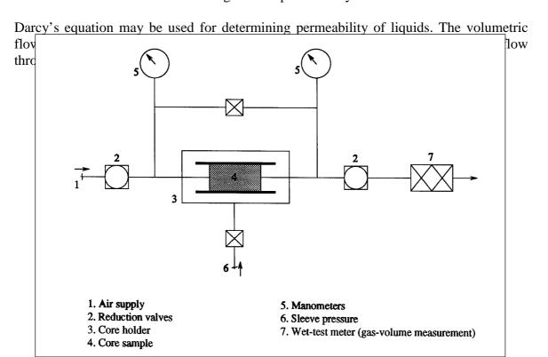
Fig. 10.3: Schematic diagram of permeameter.
