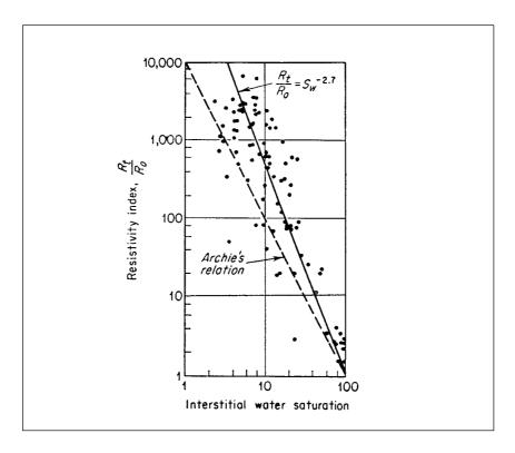
Fig. 6.4: Resistivity index versus water saturation.
