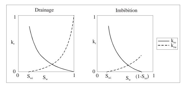
Fig. 11.1: Typical curves for oil-water relative permeability at a water-wetted system.
