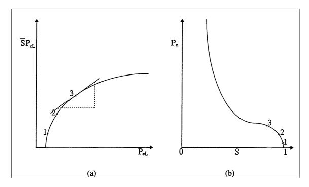
**Fig. 9.4:** Graphical differentiation of  $\overline{S}P_{cL}$  -  $P_{cL}$  curve (a) to determine S- $P_c$  curve (b).
