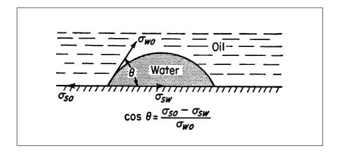
Fig. 8.1: Interfacial tensions for water-oil-solid system at equilibrium.
