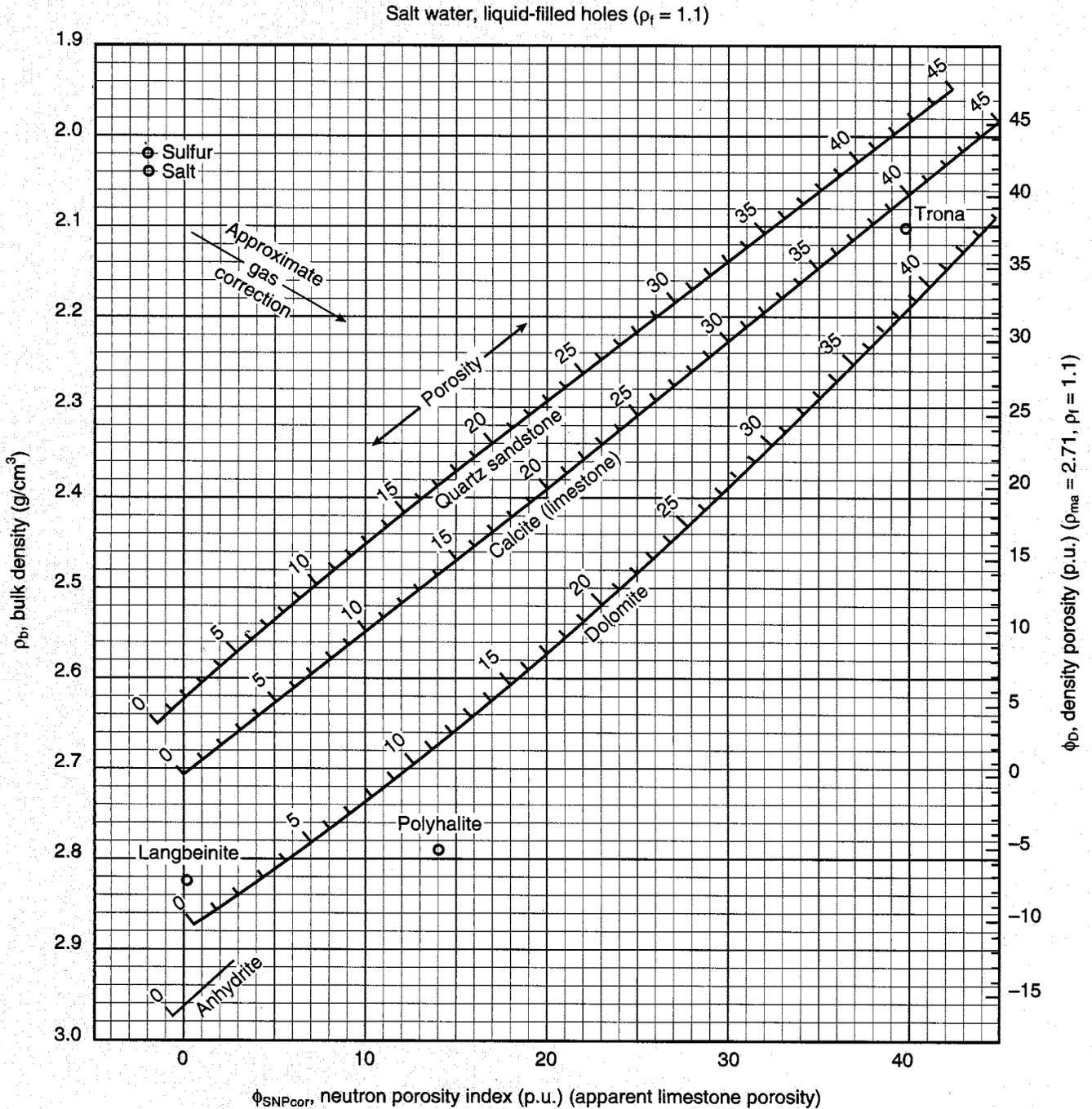
To use any of these charts, enter the abscissa and ordinate with the required neutron, density or sonic value. The point of intersection defines the lithology (mineralogy) and the porosity,  $\phi$ .
