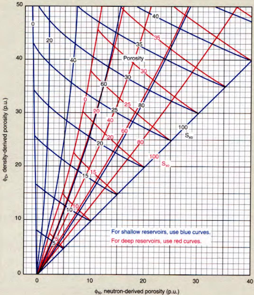
Based on reservoir depth and conditions, enter the appropriate chart with matrix-corrected porosity values. Average water saturation in the flushed zone,  $S_{xo}$ , and porosity are derived. This chart assumes fresh water and gas of composition  $C_{1.1}H_{4.2}$ , and it includes correction of the neutron log for "excavation effect."
