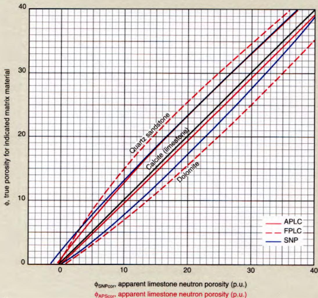
When the APS or SNP log is recorded in limestone porosity units, this chart is used to find porosity in sandstones or dolomites. First, correct the SNP log for mudcake thickness (Chart Por-15a).
