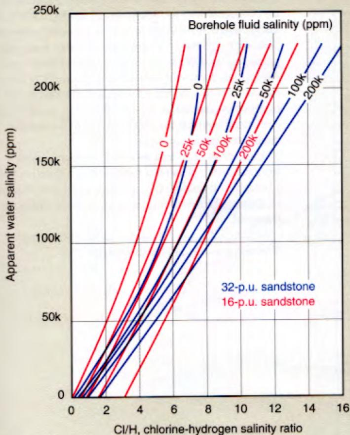
10-in. [255-mm] borehole, 7½-in. [194-mm] casing
