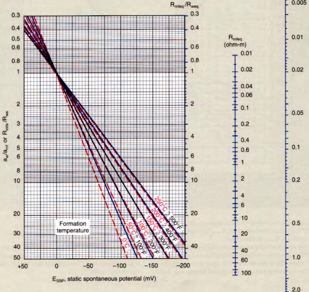
$R_w$  versus  $R_{weq}$  and Formation Temperature
