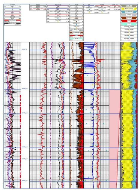
Montney interval displaying XRD calibrated shale volume
