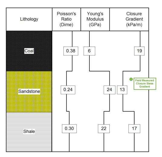
With tectonism, the closure stress base case will not match field measured data.
