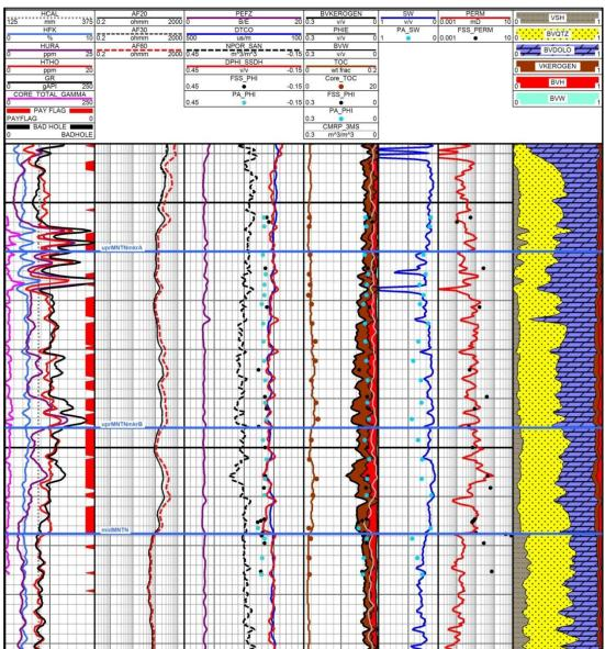
Montney interval displaying calibrated TOC weight fraction and the associated kerogen volume.
