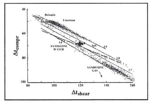
Comparison with stress test data suggest that a Poisson's ratio less than 0.179 (ΔTs/ ΔTc ratio of 1.60) reflects gas effect and not rock mechanical properties.
