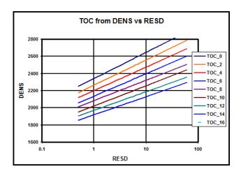
Weight fraction results calculated from logs must be calibrated to geochemical lab data using a scale and offset factor.
