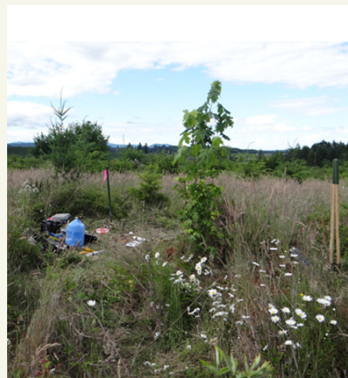
FIGURE 2: Magneto-telluric site in Oregon. A magneto-telluric system is connected to a magnetometer and two sets of electrodes to collect magnetic and electric field data. (6)
