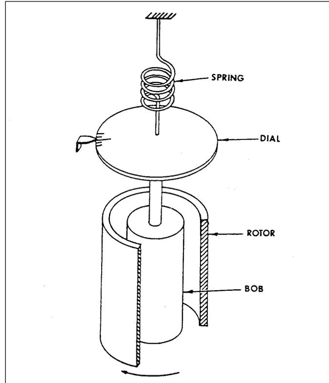
**Fig. 4.5:** Schematic diagram of the rotational viscometer.
