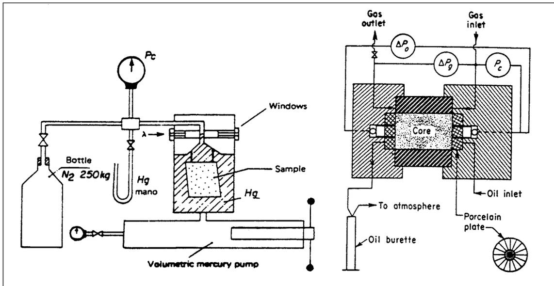
**Fig. 9.5:** Apparatus for mercury injection method.
