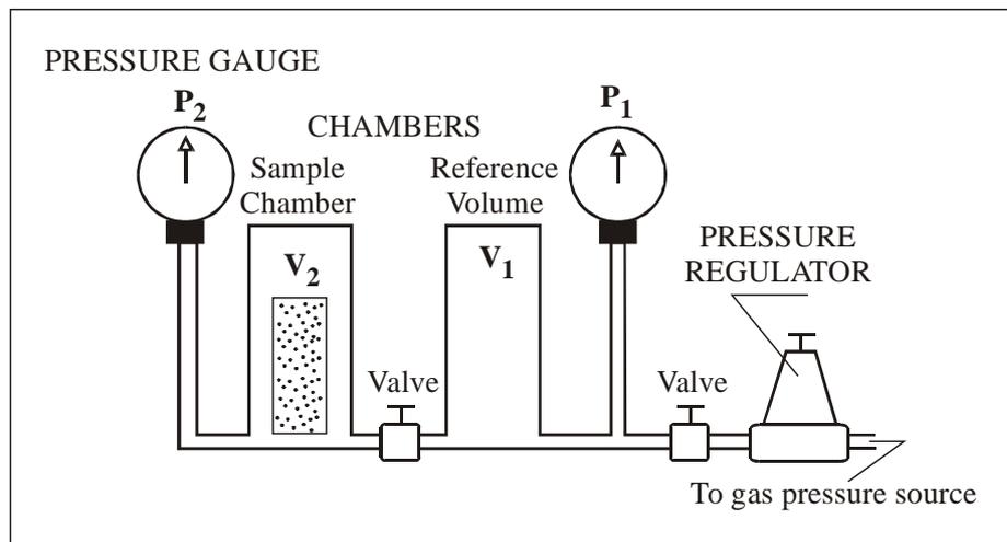
**Fig. 5.2:** Schematic diagram of helium porosimeter apparatus.
