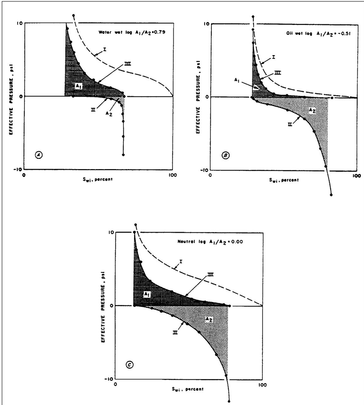
**Fig. 8.3:** Effect of wettability on the area ratio of capillary-pressure curves:
