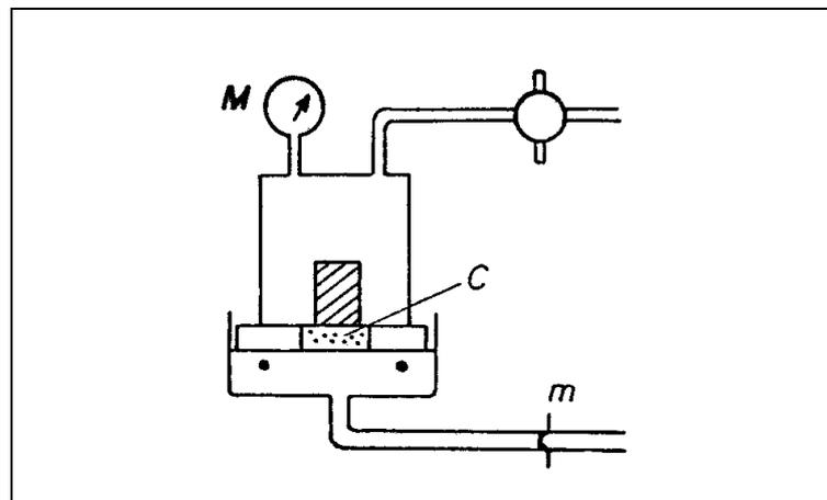
**Fig. 9.2:** The porous plate method assembly.
