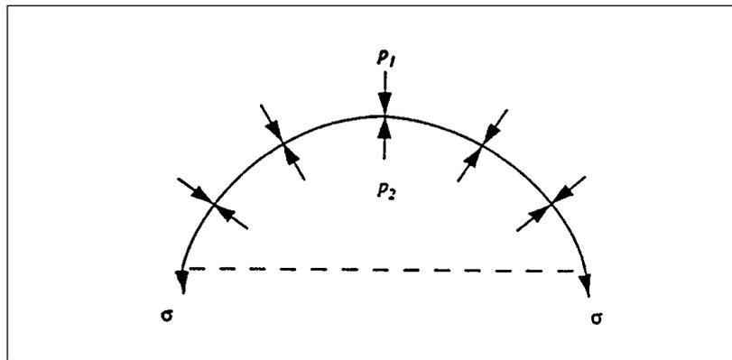
**Fig. 7.1:** Capillary equilibrium of a spherical cap.
