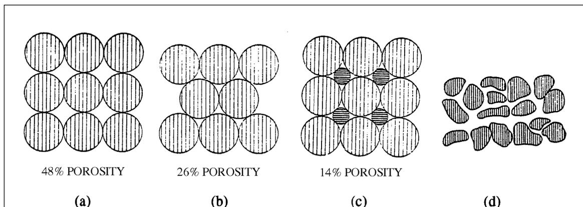
**Fig. 5.1:** Cubic packing (a), rhombohedral (b), cubic packing with two grain sizes (c), and typical sand with irregular grain shape (d).
