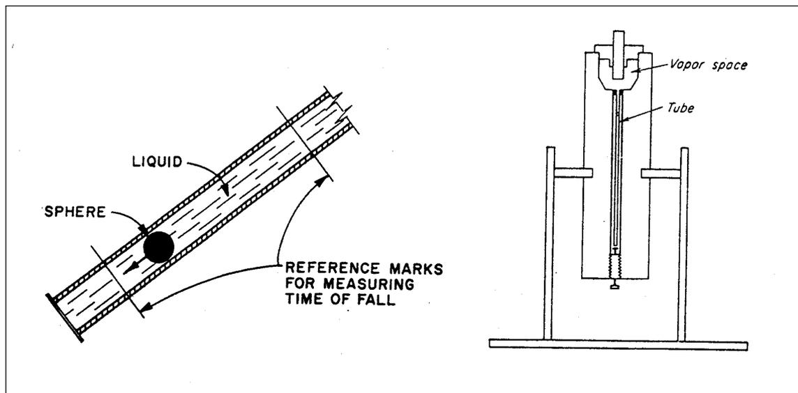
**Fig. 4.4:** Schematic diagram of the falling ball viscometer.
