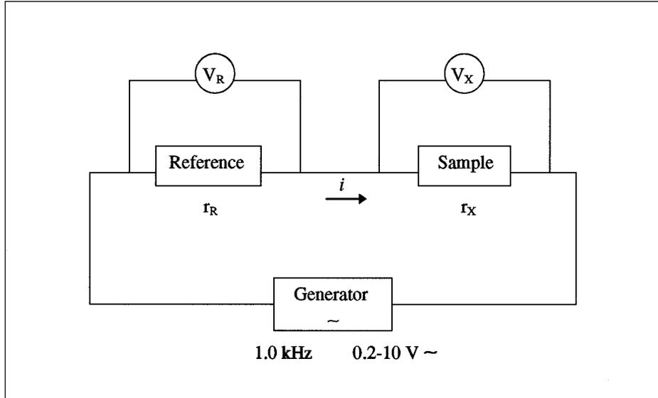
**Fig. 6.5:** The electrical circuit of resistance measurements.
