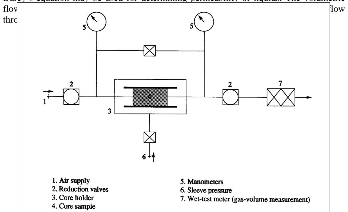
**Fig. 10.3:** Schematic diagram of permeameter.
