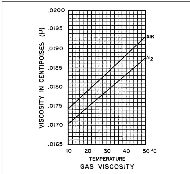
**Fig. 10.5:** Gas viscosity as a function of temperature.
